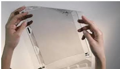
Printed Plastic OTFT array backplane
