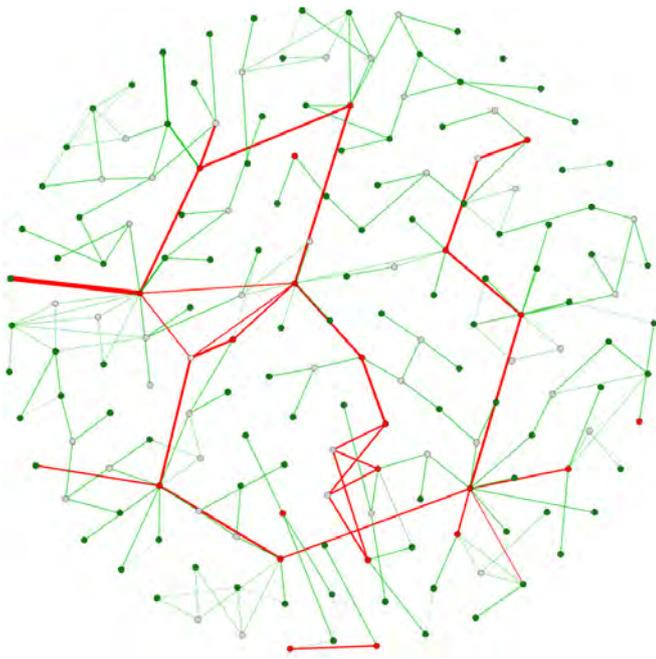
**Figure 7: Simplified part of one typical UK DNO substation network showing how National Grid 400 kV and 275 kV transmission lines (red) connect to the DNO's 132 kV and 33 kV distribution lines (green). Nodes represent substations and line junctions. Network topology is 173 nodes, 219 edges, diameter of 15 and average degree of 2.5.**
