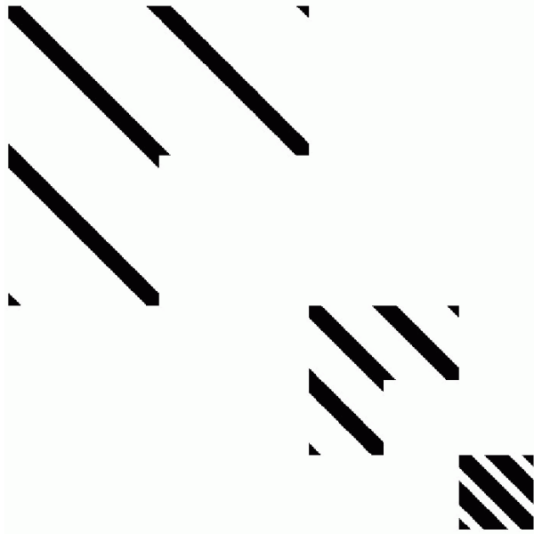
Figure 4.4: Structure of the fast wavelet differential operator
