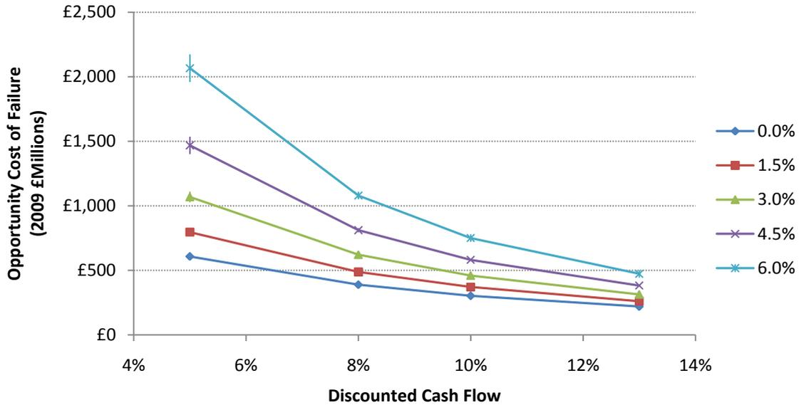
Figure 13: The cost of failure for a fleet of ADSRs (see text) that each experience exactly 5 trips per year of duration 24 hour for a 40 year life. The legend refers to the range of inflation rate scenarios that have been simulated.
