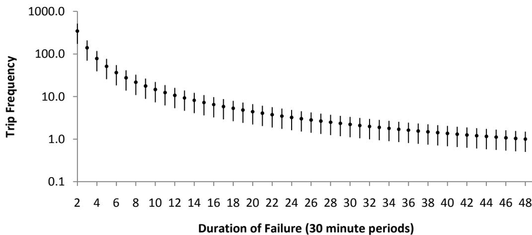
Figure 6: Frequency of shutdowns for the range 2 – 48 periods, relative to the frequency of a single 48 period shutdown. The vertical bars indicate the 50% uniform uncertainty on the mean trip frequency.
