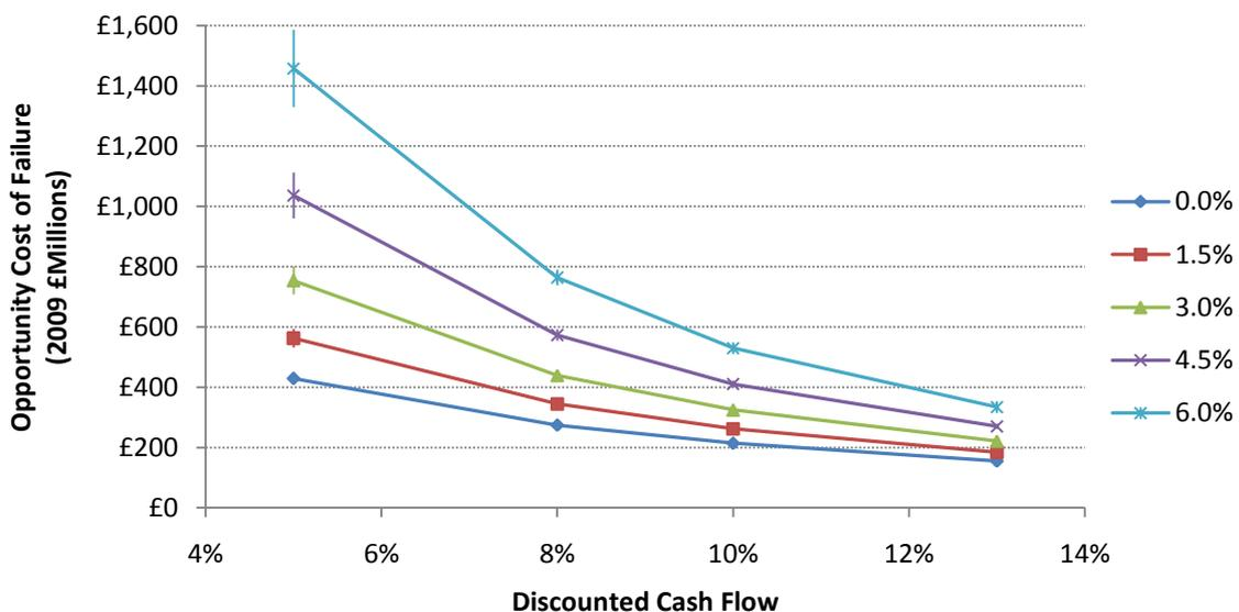
Figure 12: The cost of failure for a fleet of ADSRs (see text) that each experience a nominal unplanned accelerator system failure rate of 1% of a 40 year life. The legend refers to the range of inflation rate scenarios that have been simulated.
