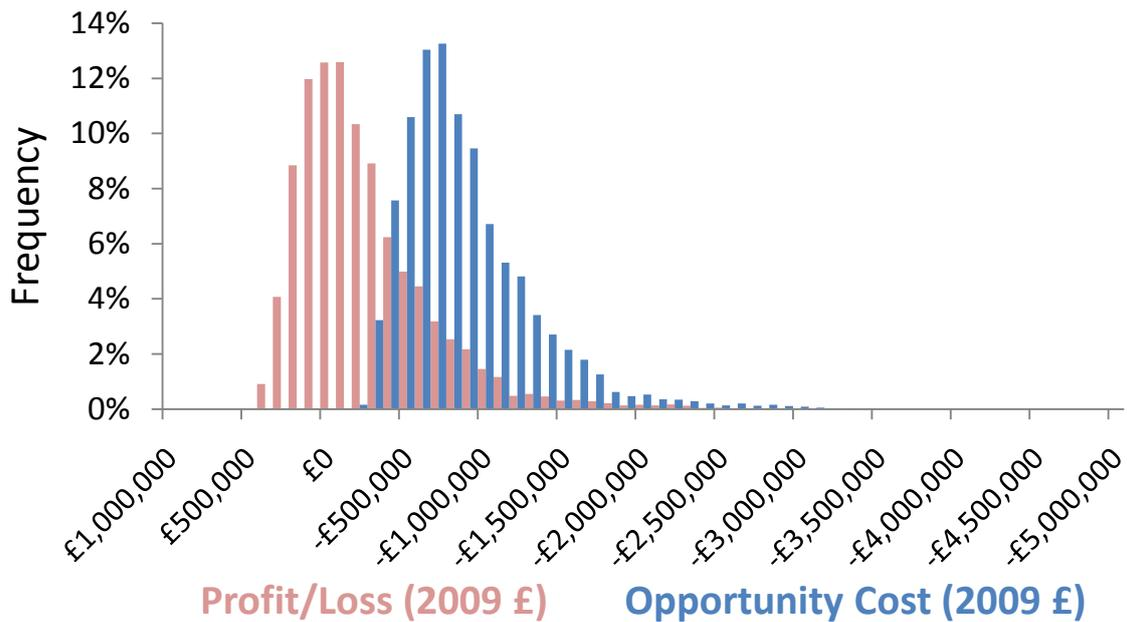
Figure 4: A frequency distribution of a 10,000 iteration simulation showing the profit/loss (light red) and opportunity cost (dark blue) of a 24 hour (48 period) unanticipated failure of an ADSR power station selling 600 MWe.
