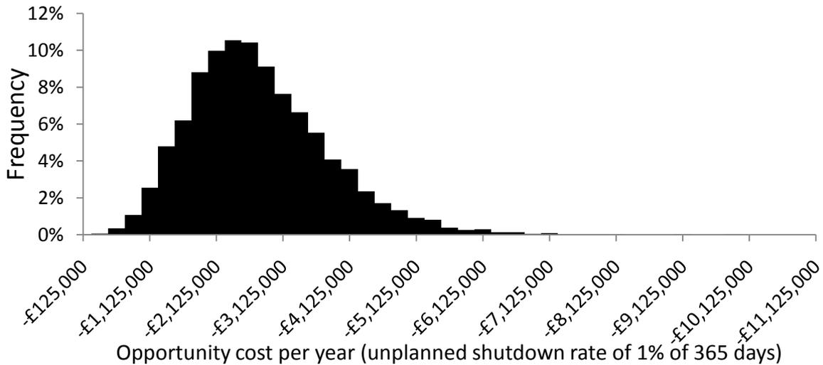
Figure 8: The opportunity cost per year to an ADSR operator for an accelerator system, which trips for a mean of 1% of the year. The mean of the distribution is £ 2,895,000 and the standard deviation is £1,045,000 in 2009 pounds.
