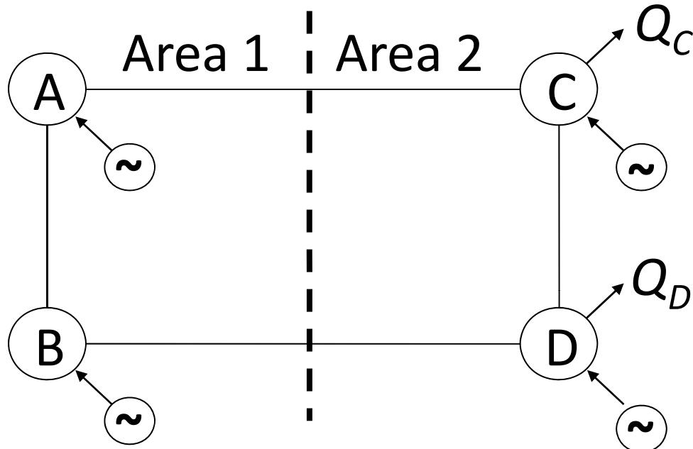
Transmission: Equal reactance, line limits = 1000 MW
