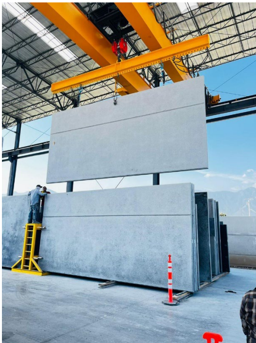
Figure 2: Finished precast concrete wall panels stored at the prefabrication plant prior to transportation and installation.
